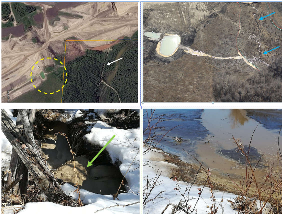
Figure 25: 18 th April 2018. High turbidity in Spring Brook (lower left – arrow points to sediment-laden flow); turbid water flowing into Beaver Pond (lower right); satellite image (top left 7 th April 201) shows probable source of sediment from temporary holding pond for runoff and/or adjacent disturbed areas (in yellow dashed circle), white arrow shows where photo of Spring Brook taken); upper right: detail of area, blue arrows show Spring Brook, flows into Weaselhead visible as tree area on lower right (April 28 th 2018)
